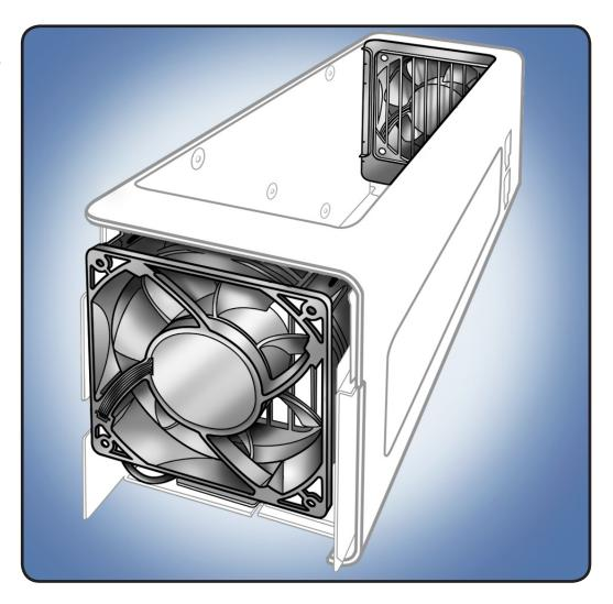
**26** Release fan cables from clips on bottom of processor cage.
